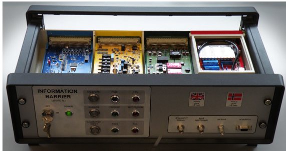
(a) A prototype information barrier for use in arms control. This would be built by the host and expected to return either a green or red light to the inspectors based on presence of nuclear material.
