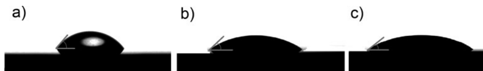
3 Drop profiles of a) PVA, b) PVA/5%MFC and c) PVA/10%MFC on Bioglass® substrates
