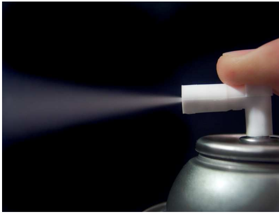
(a) Spray formation, a gas-liquid flow.
