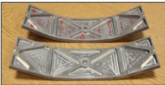
Figure 8.5: Illustration of (i) the visual profile and (ii) comparison of the profile between CAF and CWBSFA workpieces.
