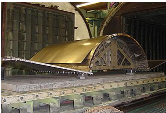
Figure 2.1: Creep age forming workpieces. (a) The world's largest commercial aircraft A380 wing panel [43], (b) Gulfstream G-5 wing skin [43], (c) GKN aerospace engine inner fixed structure [51].
