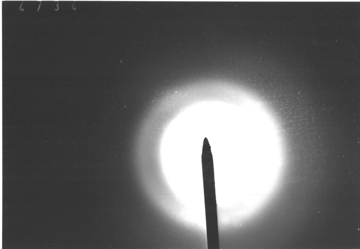
Fig.4.36 Electron diffraction pattern of the same film of Fig.4.34 and 4.35.
