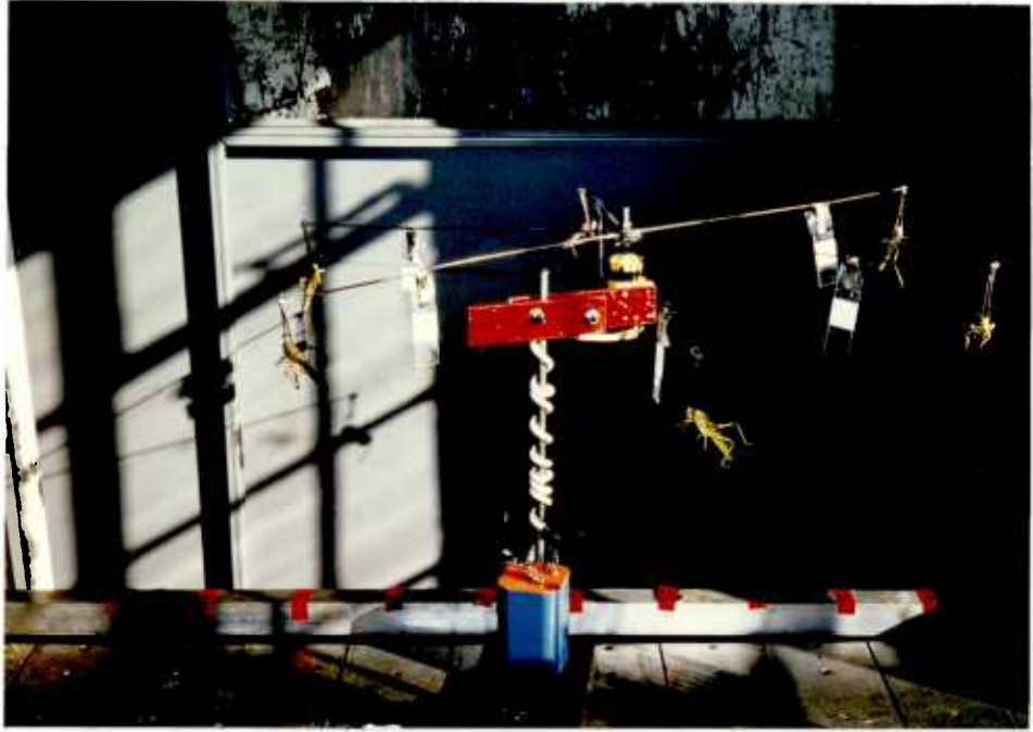
Plate 6 A stand on which locusts and glass slides were rotated in a cloud of spray droplets.
