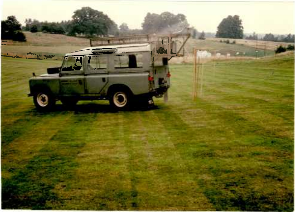
Plate 1 Multiple - disc (15 discs) sprayer fixed to a Land - Rover
