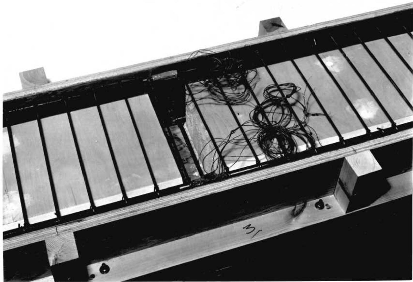
Plate 5.1 Channel Section with Single Stirrup Reinforcement.
