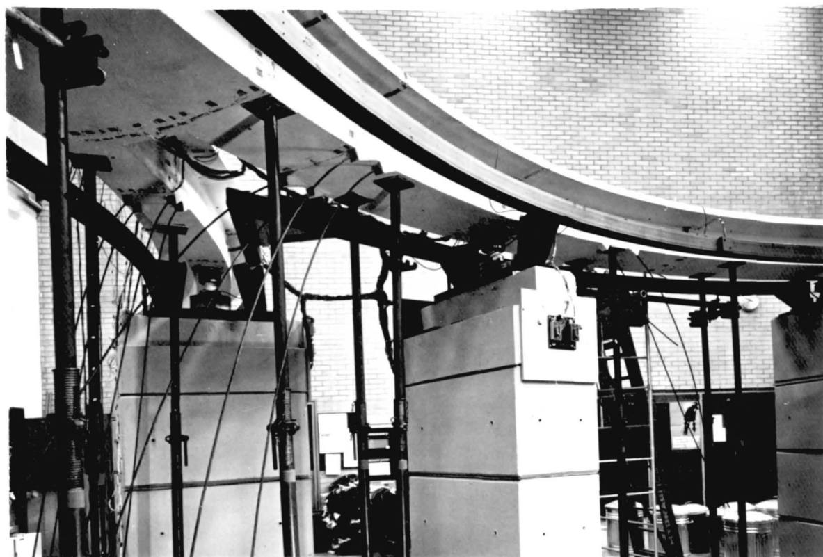
Plate 4.1 The Microconcrete Bifurcated Bridge Model
