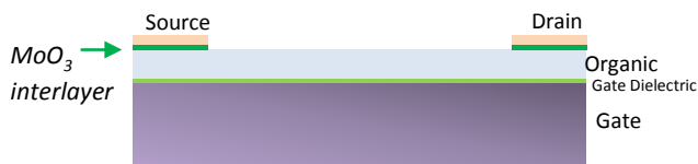
Fig. 2.18 Schematic of a top-contact bottom gate (TCBG) OFET with a thermally evaporated MoO_3 interlayer
