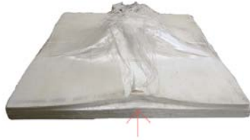
Figure 15: Full Dyneema® HB26 panel impacted at 1410 m/s by a steel FSP.
