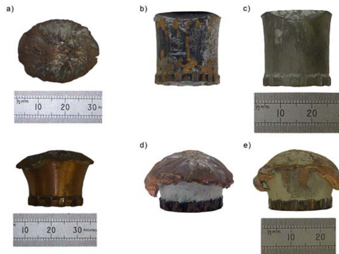
Figure 5: Photographs of the post-mortem projectiles: a) The copper FSP fired into the catcher box at 1 km/s (top view and side view); b) St FSP, Dyneema ® HB26, V_s=1008 m/s; c) St FSP, Spectra ® 3124, V_s=1016 m/s; d) Cu FSP, Dyneema ® HB26, V_s=1047 m/s; e) Cu FSP, Spectra ® 3124, V_s=1027 m/s.
