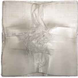
Figure 15: Full Dyneema® HB26 panel impacted at 1410 m/s by a steel FSP.
