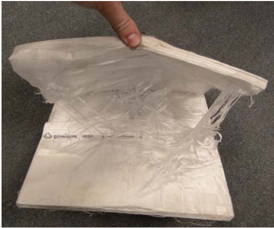
Figure 24: Full Dyneema ® HB26 panel impacted at 609 m/s with a steel FSP.
