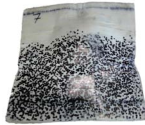
Figure 16: Full Spectra® 3124 panel impacted at 466 m/s by a copper FSP.
