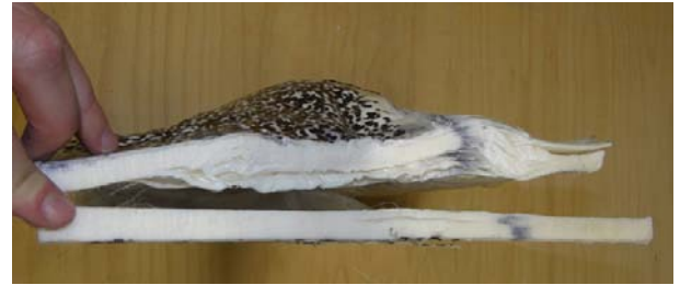
Figure 25: Full Spectra 3124 panel impacted at 640 m/s with a steel FSP (the two split parts being held together by the author).
