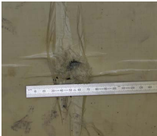
Figure 13: Magnified view on the Dyneema® HB26 panel impacted at 509 m/s by a steel FSP.
