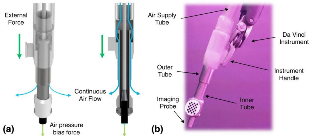
**Figure 1** (a) Computer-Assisted Drawing (CAD) model of the proposed drop-in mount (left) and its section view (right) demonstrating the air flow path; (b) fabricated instrument handled by the Da Vinci Endowrist Needle Driver.
