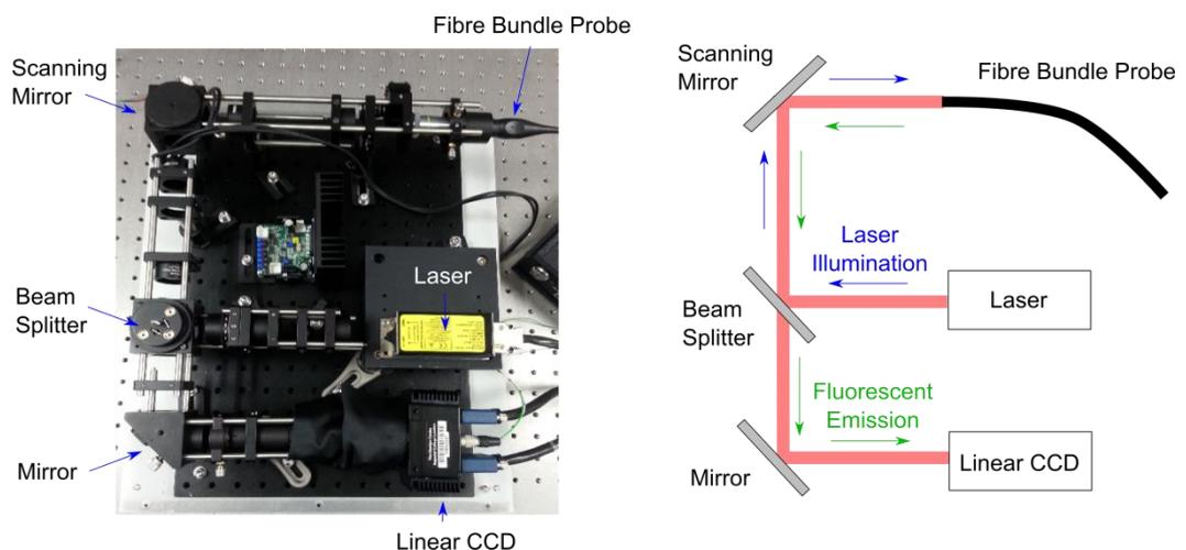
**Figure 2** Photograph and schematic of the endomicroscopy imaging system, showing only the key components. Intermediate relay optics, and optomechanics are not shown for clarity.
