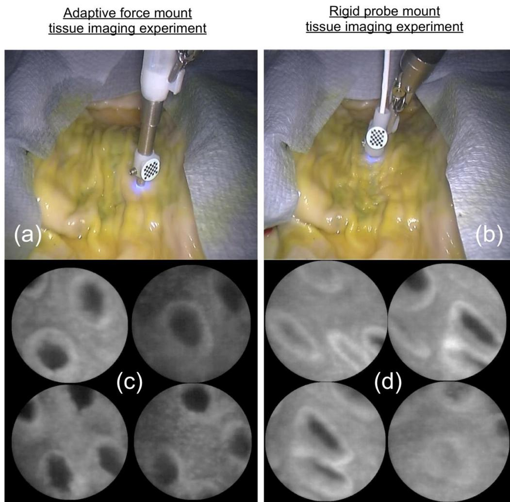
**Figure 4** (a-b) Snapshots during the tissue task where the users had to scan, with the adaptive robotic mount (a) and a rigid mount (b), a large curved 3D surface and acquire consistent microscopy images. (c-d) Indicative microscopy images sampled during the tissue task with the adaptive probe (c) and the rigid probe (d).
