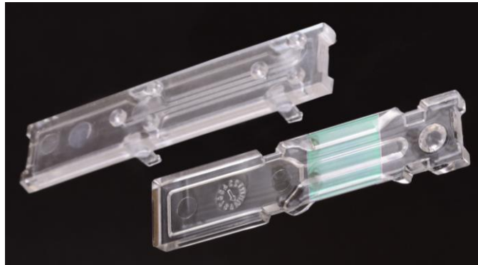
Figure 1. Photograph of an injection molded chip coated with dielectric thin film stack and a flow cell, the latter being prepared by two-component molding.
