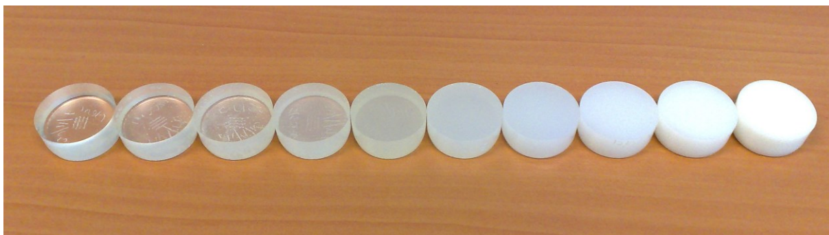
Figure 2.1: Epoxy phantoms of increasing density from left to right.
