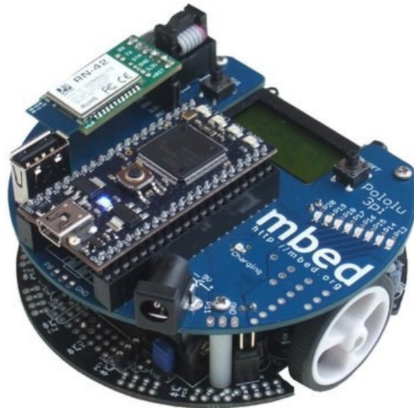
Figure 15. 3pi robot with mbed controller. The robot is powered by four AAA batteries. It is controlled by ATmega328 microprocessor. The internal voltage regulator boosts the motor voltage to 9.25V, guarantees its speed performance.
