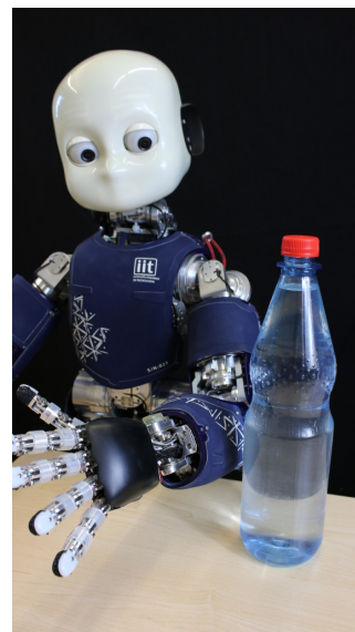
Fig. 1: The humanoid robot iCub . Its movement is obstructed by an unexpected obstacle, which decreases the tracking performance of a desired trajectory. We reduce the tracking error by learning the torque control to compensate the contact.
