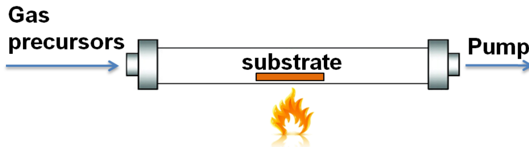
Figure 3-1: Schematic of a typical CVD system
