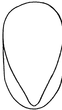
Cross section of levitated metal with slag attached
