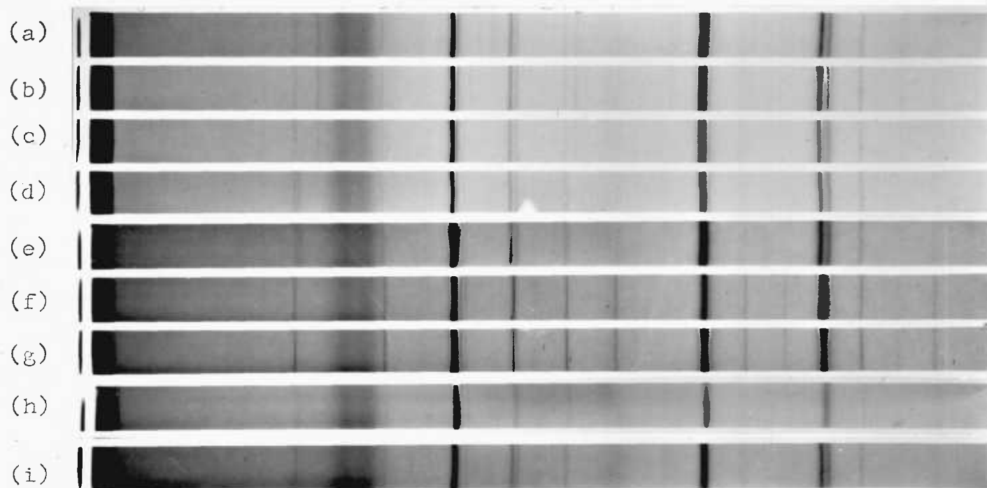
Fig. 24 Guinier photographs of stannites quenched from the temperatures:
