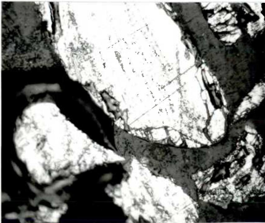
Fig. 46 Photomicrograph of leach residue 41.1% copper dissolved. ( X 300 )
