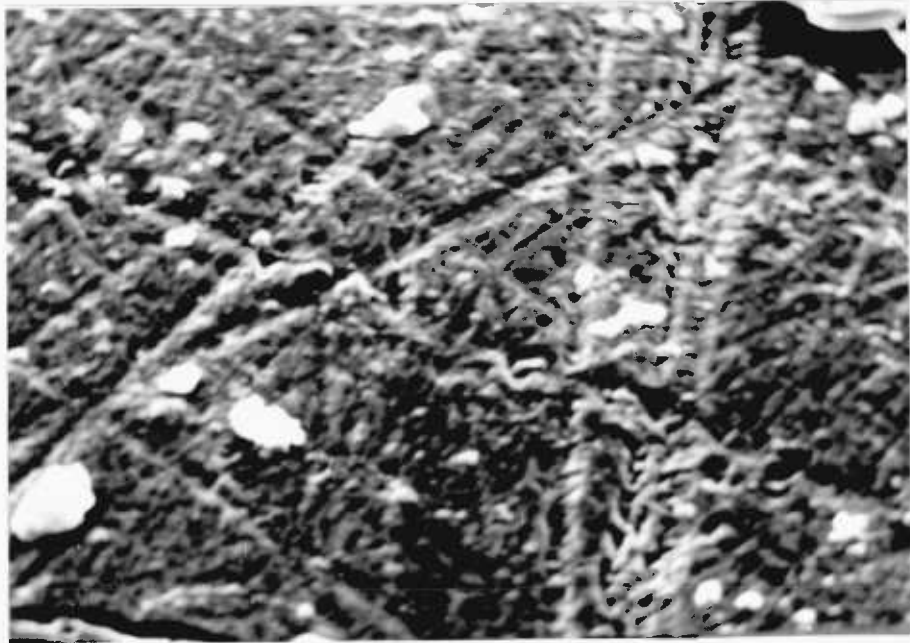
Fig. 52 Scanning electron micrograph of a partially leached specimen. ( X5000 )
