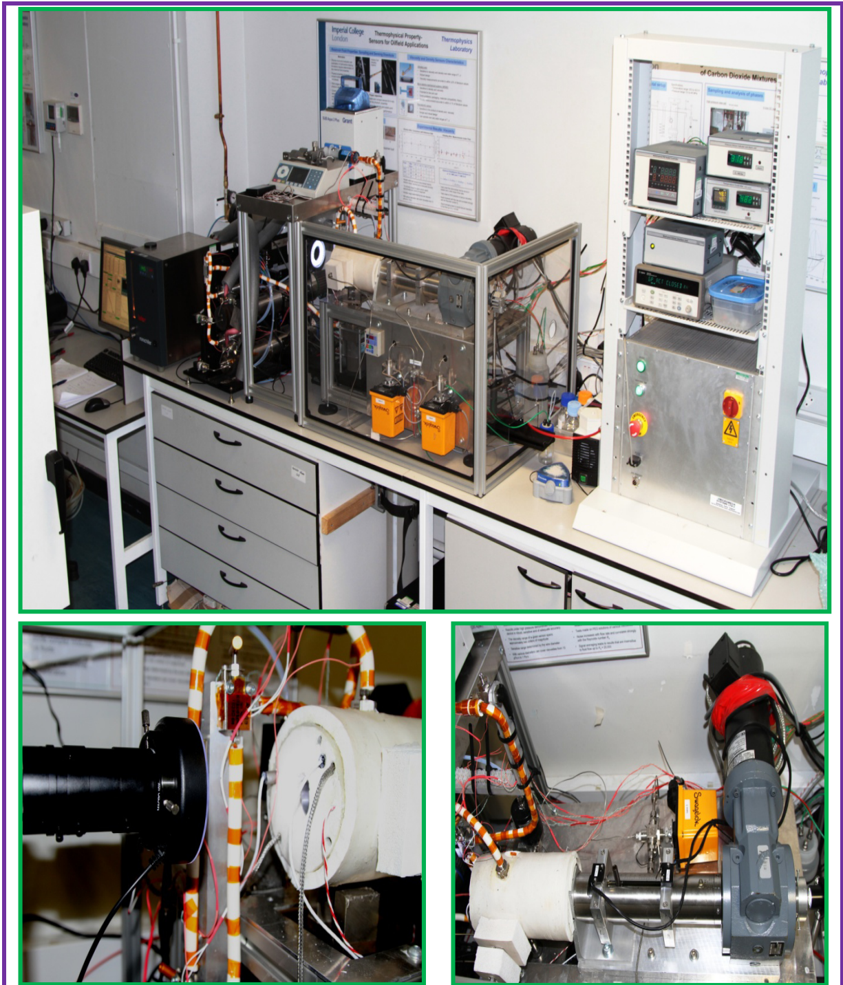
Figure 4.3. Pictures showing the synthetic apparatus setup located in the chemical engineering department, ACEX building, lab 424. The top picture represents the entire apparatus including the variable volume cell assembly, a rack holding the servo controller and other instruments, the Quizix pumps, the chiller and fluid system. The bottom left picture shows the CCD camera used and the front of the equilibrium cell. The bottom right picture represents the variable volume equilibrium cell (top view) combined with the servo motor, gear box, limit switches and the encoder.
