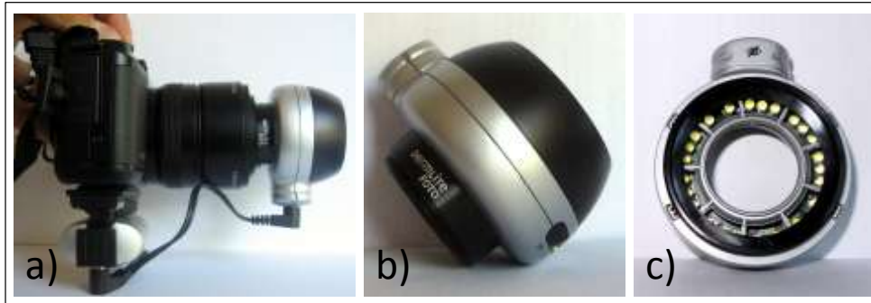
Figure 4.1 (a) G10 Cannon Camera shown with dermoscopic attachment. (b) DermliteFOTO® dermoscopic lens detached from camera. (c) DermliteFOTO® ring light attachment for macroscopic imaging.
