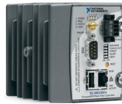
Figure 1.7 NI cRIO-9014 Real-Time Controller
