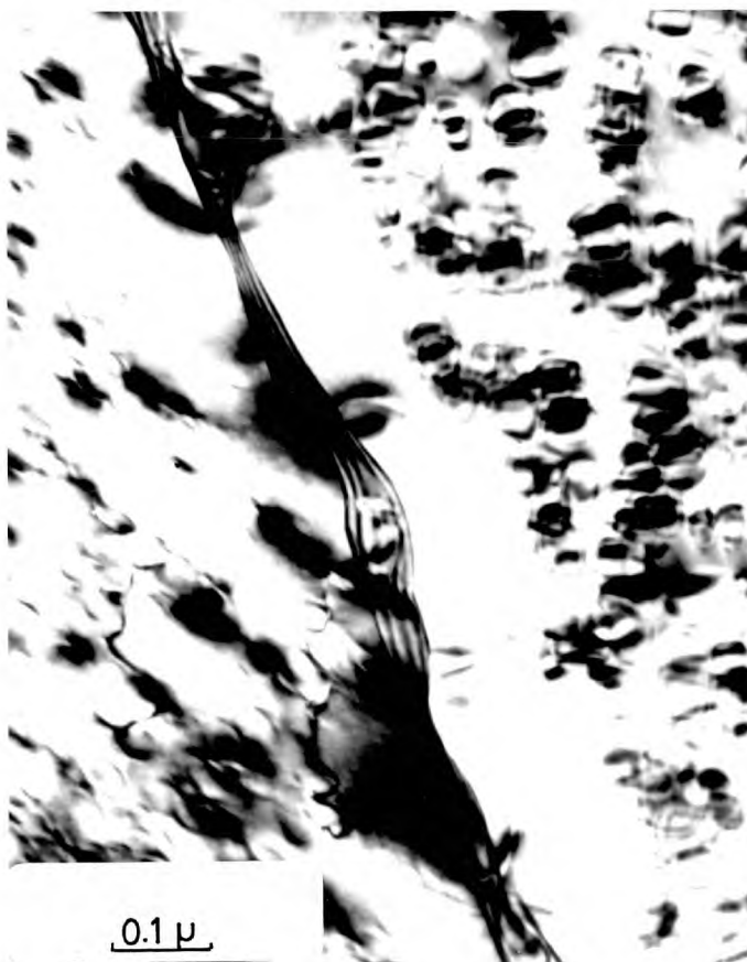
Fig.4.1.10. Alloy B. aged 43 hours at 700°C. Foil orientation: L.H.S. (211) R.H.S. (110). Operating reflections: L.H.S. (T11) R.H.S. (200).
