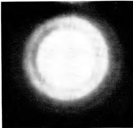
Figure 3(a). Transmission electron diffraction pattern from a deposit containing 75% neon and 25% argon at 7 °K (50 keV electrons).
