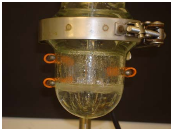
Figure 2. Photograph of phase separated emulsion (water to oil phase (1:1 styrene/poly(ethylene glycol) dimethacrylate) volume ratio 80:20) demonstrating that oleic acid alone is not a suitable emulsifier to stabilize w/o HIPEs
