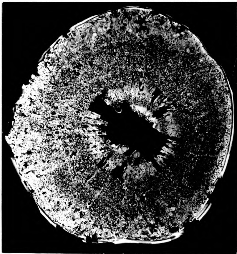
Figs. 4.8.1 and 4.8.2 Sections of stones \alpha and \alpha' in the plane of their longest axes photographed between crossed polaroids to show the constituent crystallites and by transmitted unpolarized light to show the bubble structures. Magnification: 3.25 \times 3.25
