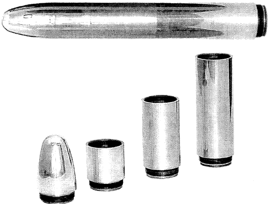
Figure 2.9: Photograph of the assembled non-instrumented model; Nosepiece and various interchangeable cylindrical afterbody segments.
