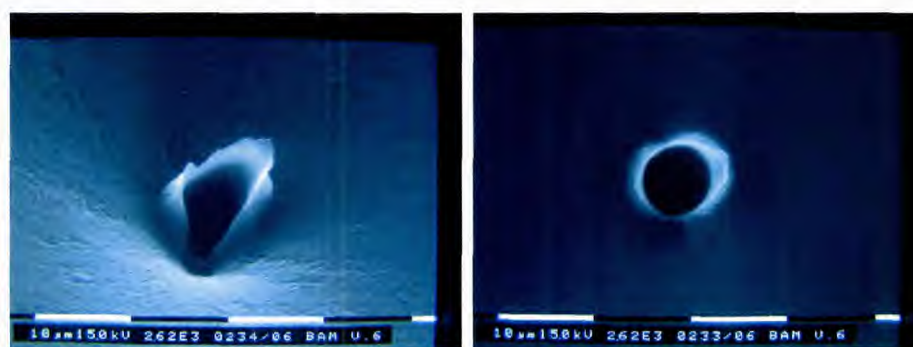
Figure 66: Representative SEM micrographs of 2.5 wt% CNT in PEEK matrix after fibre pull-out
