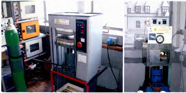
Figure 29: Images of the hot presses used for compression moulding
