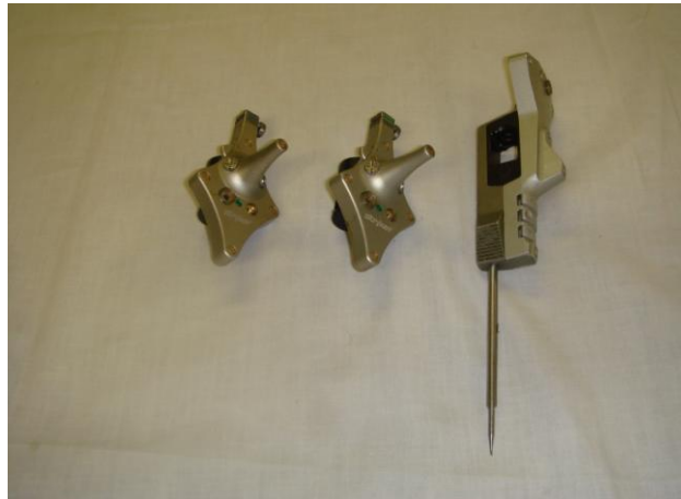
Figure 21 The Femoral and Tibial Trackers and Pointer.
