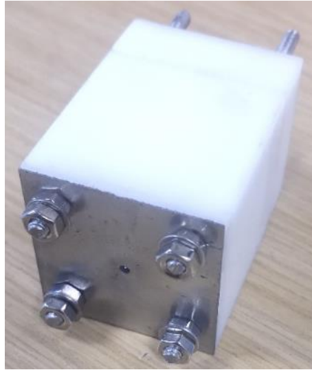
Figure 8: Thruster housing for a single emitter tip, comprised of an extractor plate with a single aperture and a porous reservoir.
