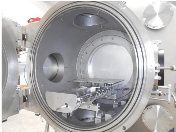
Figure 6: The vacuum system in the David Fearn Electric Propulsion Laboratory at the UoS.
