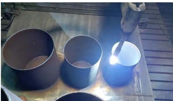
(a) WAAM CHS for compression tests
