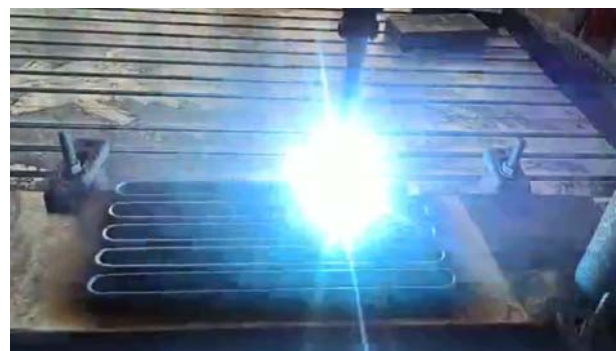
(b) WAAM oval tubes with flat sides for tensile coupon tests
