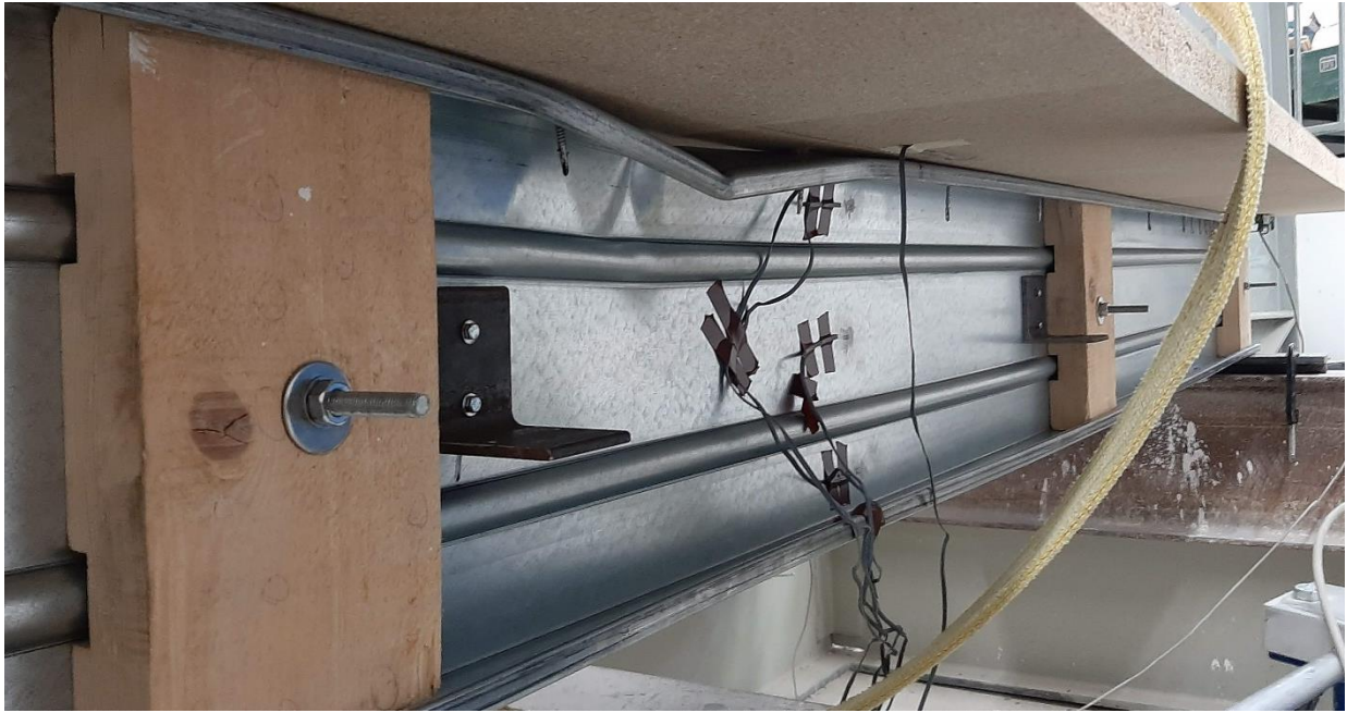
Fig. 14. Failure of specimen No. 3 – Distortional buckling within the constant moment region
