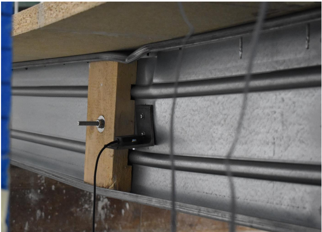
Fig. 15. Failure of specimen No. 5 – Local buckling, with some distortional contribution, within the constant moment region
