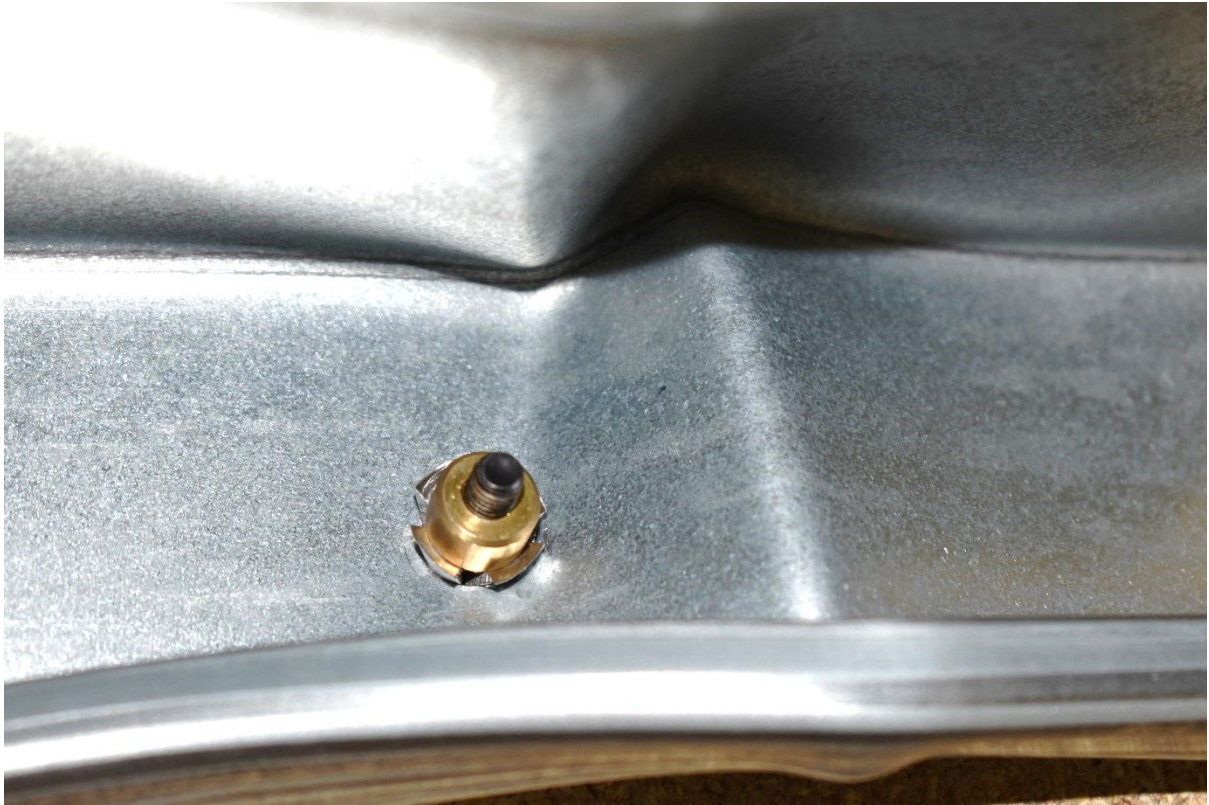
Fig. 16. Failure of specimen No. 5 – Local buckling, with some distortional contribution, adjacent to the connector
