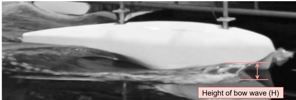
Figure 10: Flow around the hull at draft = -16cm and speed = 2m/s with the bow wave highlighted.
