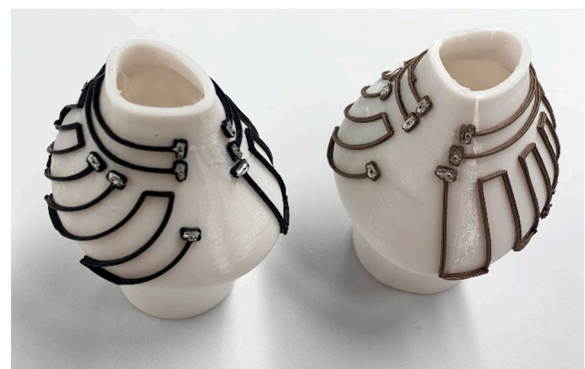
Fig. 19. Conductive traces conformally printed onto vase-like doubly curved substrate. Left) Carbon-based trace; and Right) copper-based trace.
