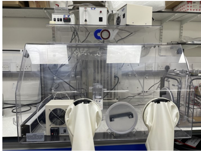
Fig. 5.6 Environmental Control in a Coy Laboratory Products Humidity-Controlled Glovebox
