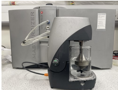
Fig. 6.2 Photograph of the Mastersizer. This apparatus is used for the analysis of particle size distribution.
