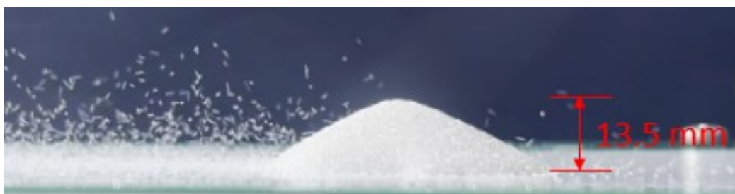
Fig. 6.1 Measurement of the thickness h of tested particle on the ETW board.
