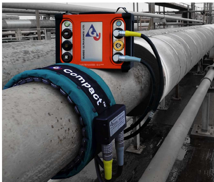
Figure 2.9: An example of guided wave testing inspection setup [19].
