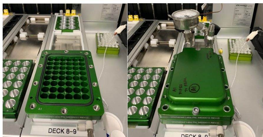
Figure 14 A 48 well Deck Screen Pressure Reactor (DSPR).
