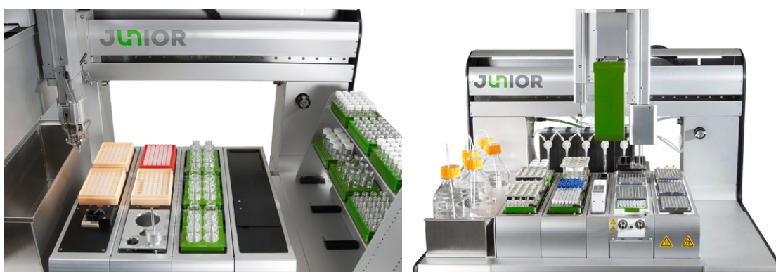
Figure 13 Pictures of a) Unchained Labs “Junior” Power Dispensing Robot (left) and b) Unchained Lab “Junior” Liquid Handler and Reactor. 102
