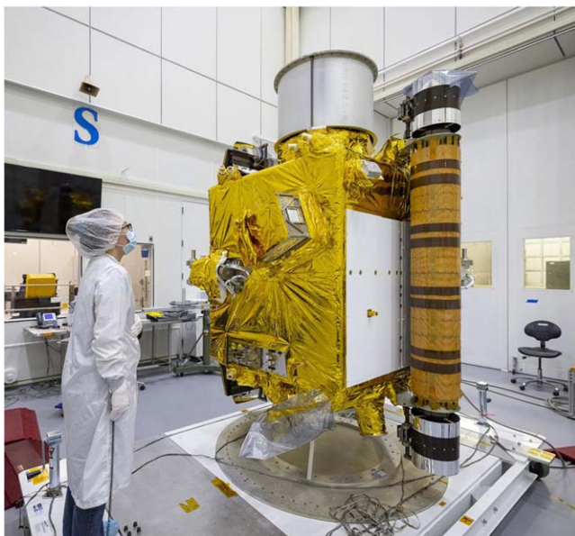
Figure 1. The DART spacecraft in 2021 September, during the pre-ship inspection at the Johns Hopkins Applied Physics Laboratory. In this image, the NEXT-C ion-propulsion engine is at the top of the spacecraft, one of the rolled-up ROSAs is on the right side, and LICIAcube is contained on the gold-colored blanketed spacecraft side. In this position, DRACO is not visible as it is pointing at the floor. The main structure of the spacecraft is roughly a cube with dimensions of about 1.3 m, from which other structures extend to result in measurements of roughly 1.8 m in width, 1.9 m in length, and 2.6 m in height.
