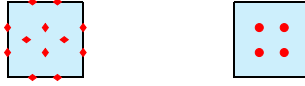
Fig. 1. The degree 2 RTCF tensor product element (Raviart-Thomas H(\text{curl}) elements on quadrilaterals, [Raviart and Thomas 1977]) (left) used in Listing 1. The RTCF element is an example of a tensor product element in 2D, which depending upon the orientation of the DOFs on the edges, can be used for either H(\text{div}) or H(\text{curl}) problems. The right displays a similar example for the DQ element, which is an L^2 -conforming tensor product element in 2D, and is necessary to form the stable pair for the mixed Poisson problem.
