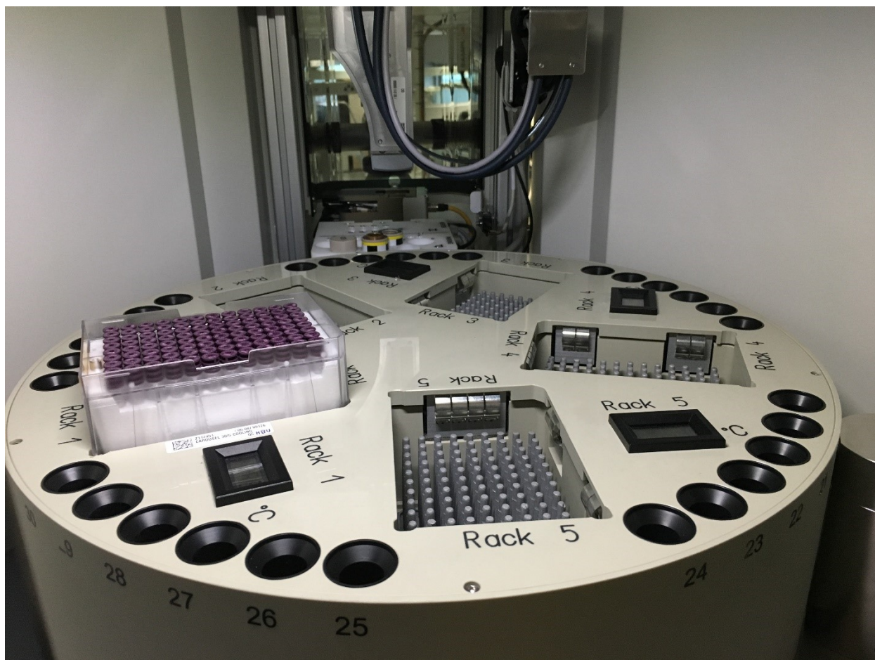
Figure 20. Photograph showing the NMR spectroscopy racks used to analyse the samples in this thesis. NMR – nuclear magnetic resonance.
