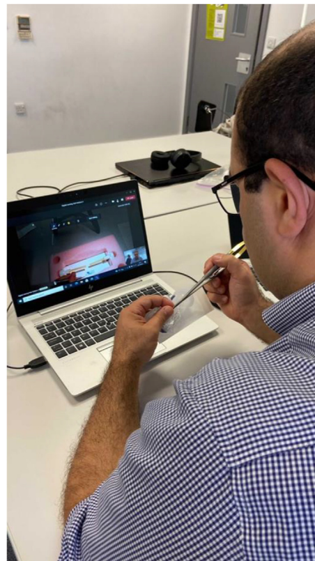
Fig 3. The trainer is able to see their trainee's point of view, through a camera on the head-mounted display (HMD).
