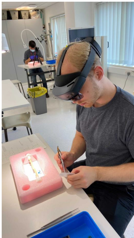
Fig 2. Participant wearing HoloLens head-mounted display (HMD). They are able to see the vessel and jig and their trainer superimposed over their field of vision.
