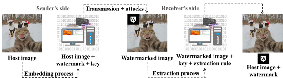
Fig. 11 A working illustration of a blind watermark extraction process
