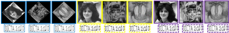
Fig. 12 Robustness illustration of a robust watermark when exposed to different attacks. Solid blue, yellow, and purple boundaries contain the watermarked images under rotation attack at 45°, Gaussian noise (GN) at 0.001, and JPEG compression with a quality factor (QF) of 40, respectively. All dashed borders represent the extracted watermarks from the attacked watermarked images. This illustration is achieved using Sharma et al.’s methods in [99]. Best viewed when zoomed in
