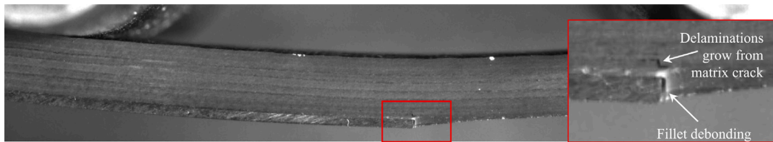
Fig. 18. A specimen with a straight edged adherend immediately before the sudden load drop. Delaminations can be seen to grow from a matrix crack and debonding of the adhesive fillet from the adherend edge is visible.
