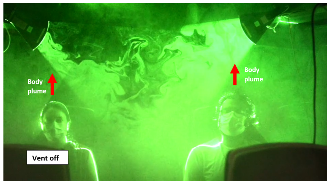
Figure 11. Snapshot of flow visualisation experiment at the middle of carriage during unventilated conditions. Red arrows indicate direction of persistent air flow.
