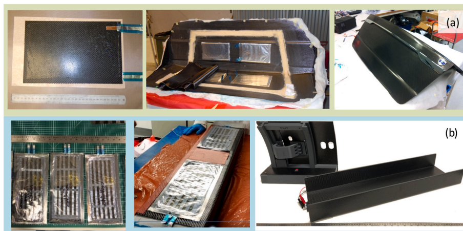
Fig. 11. Multicell structural supercapacitor components (a) STORAGE Volvo S80 bootlid assembled from four stacks, each of four cells, within a CFRP skin [156]; (b) SORCERER C-beam showing individual cells, two stacks of four cells being integrated into the C-beam and connected to a desktop scale model of an aircraft door [157].
