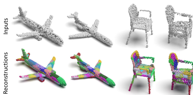
Fig. 11 Rigid inter-class (within category) regional shape correspondence. Correspondences on 64 local patches reconstructed from 64 different capsules are visualized with color coding. Regions under correspondence are assigned identical colors. No supervision signal is utilized for correspondence estimation
