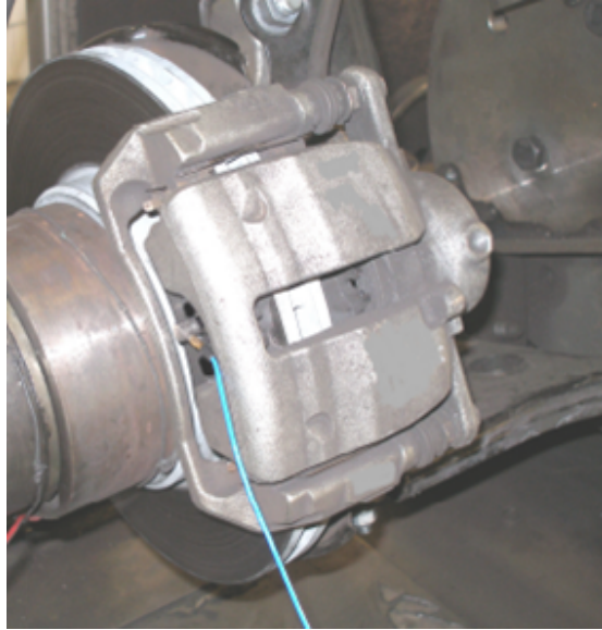
Figure 1: Brake system with accelerometer based on the backing plate of the brake pad mounted on commercial brake test rig.
